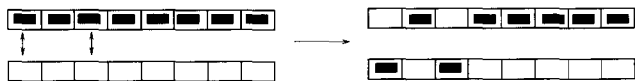
Fig. 4. The uniform crossover operator for real encoded parameters. Each block denotes a specific parameter. In DGΩ, each parameter represents a lower or upper bound of a distance restraint.
